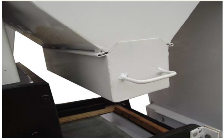
Settling chamber for collect the heavy light impurity
