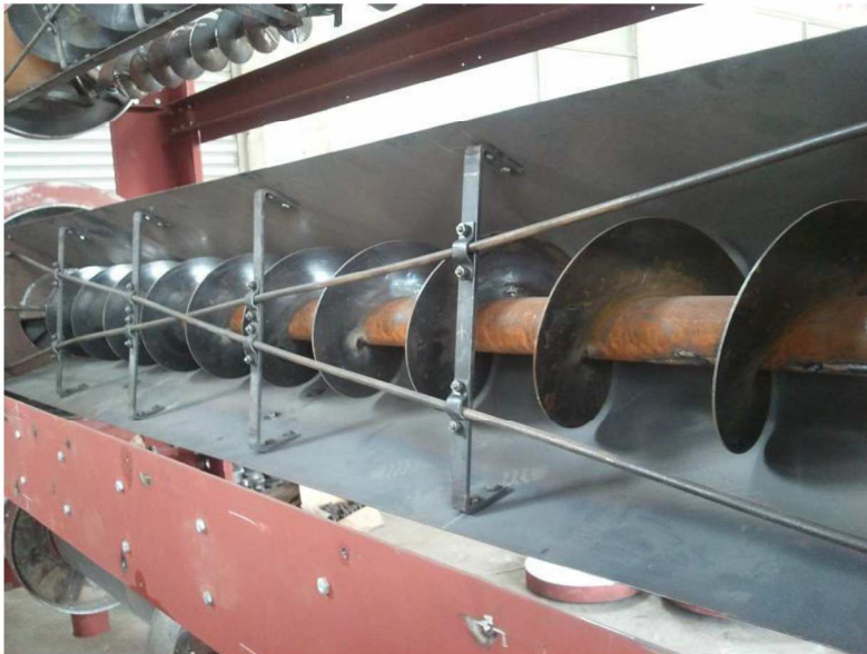
Screw Conveyor that inside of cylinder
