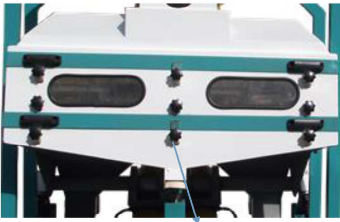
Through-hole handle to fasten sieves
