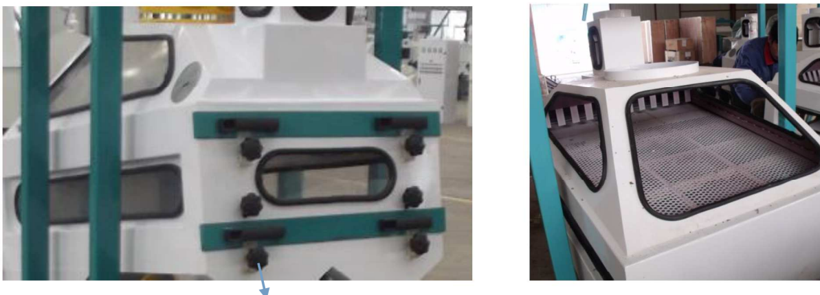
Through-hole handle to fasten sieves
