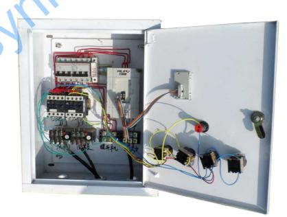
We installed frequency inverter in power control box which can adjust sieve table vibrating speed.
