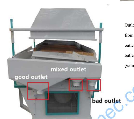
Outlets of gravity separator, from left to right is good outlet (heavy grain), mixed outlet and bad outlet (light grain)
