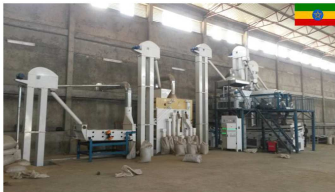
8T/H Soybean, red kidney bean, lentil, chickpea and 6T/H sesame cleaning plant in Ethiopia
