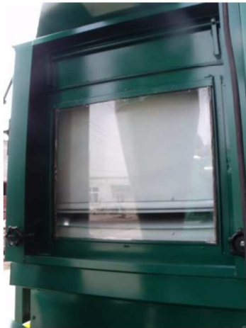
Mirror of aspiration chamber for observation
