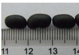
Rubber ball for sieve clog cleaning
