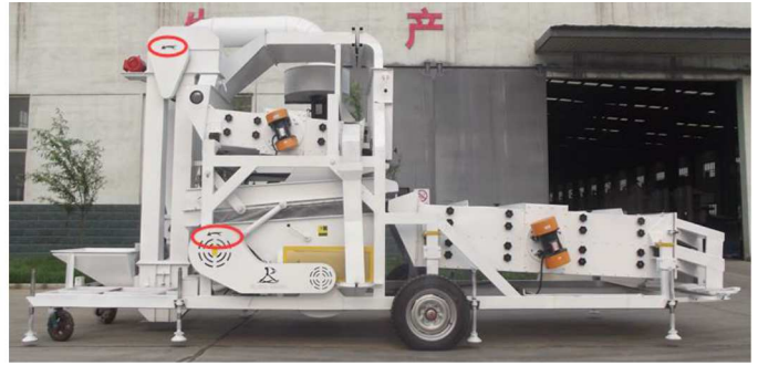
Please check the machine rotation before operation. Make sure motor rotation direction is same as marked arrow.
